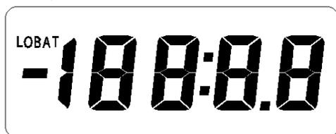
continuously. At this point there is ample power in a 9V alkaline battery to operate the tach for several more hours without backlight but the battery should be replaced on landing.
