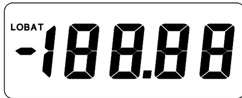
mean that the battery needs to be replaced. When the battery voltage falls too low to operate the instrument, the LO BAT legend will continuously flash on and off as a warning. When this first happens, there is still sufficient life in a 9V alkaline battery to operate the instrument for almost 2 hours.
